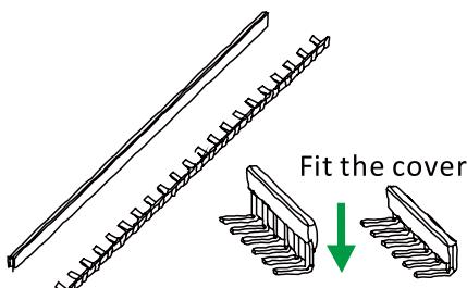
8. Fit the busbar and connect incoming/outgoing cables as required.
