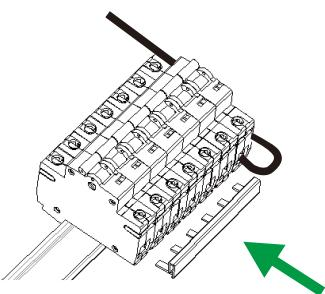
9. Ensure all the connections are fully tightened as specified below.
