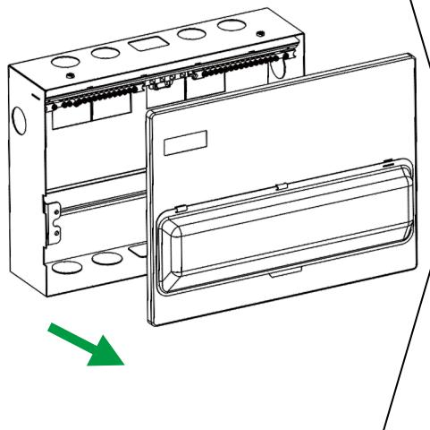
2. Remove the minimum amount of relevant knockouts for the incoming/outgoing cables.
