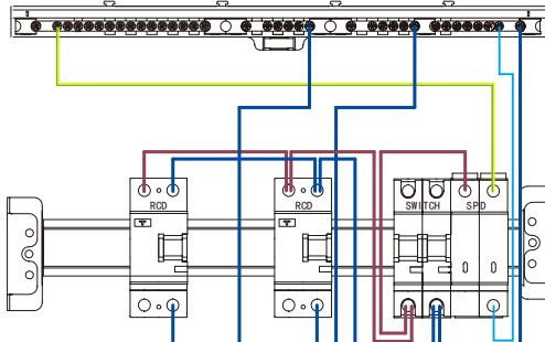
6. Fit the device by clipping onto DIN rail.
